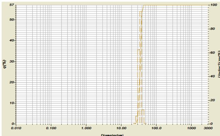
A median particle size of 35 micron and a particle size distribution of less than 1.4 ( $d_{60}/d_{10}$ ) show a lack of fines and result in high efficiency at low back pressure.
