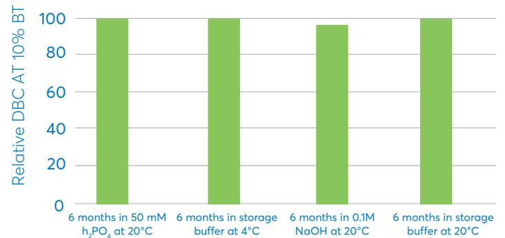
Dynamic binding capacity is maintained under various storage conditions.
