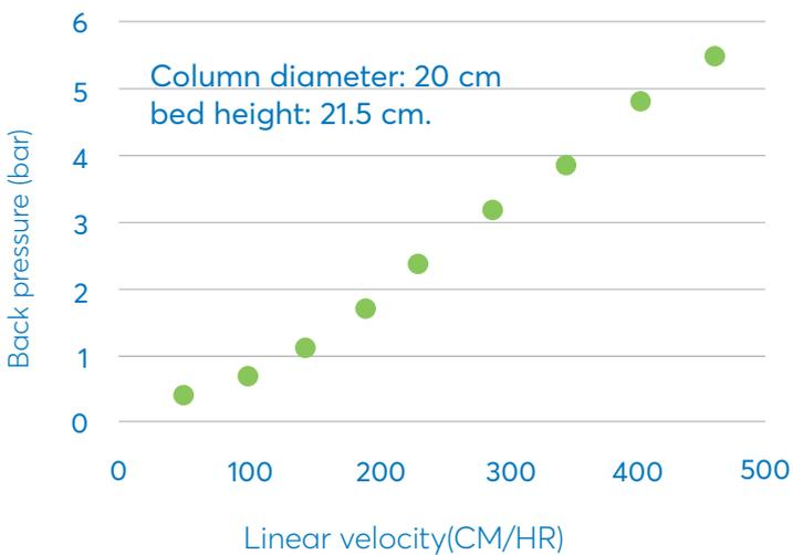
The linear behavior of the pressure-flow curve indicates no resin compression.
