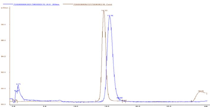
The conductivity peak shows an efficiency of 11,061 plates/meter at an asymmetry of 1.15.
