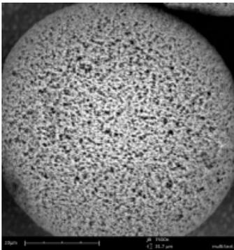
The average pore size of the beads is 500 Å, providing an exclusion limit of  $1 \times 10^6$  Dalton
